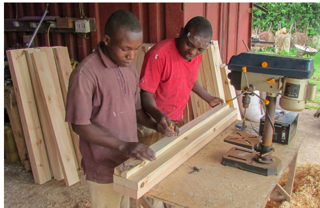
Making window frames
